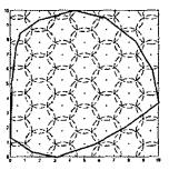
Fig. 3. Covering a convex region using a minimum number of disks
